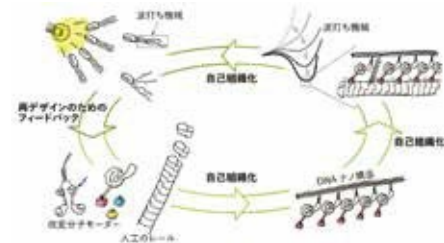
Figure 3. Example of an autonomous micro-robot with a hierarchical structure, which is our goal (Furuta et al., Curr Opin Biotechnol 2017).
